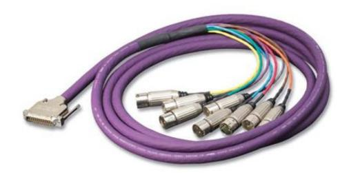
Suitable for Analogue audio output this cable assembly is wired to the Tascam DTRS convention. Belden 7880A low-capacitance, individually screened, 110 Ohm eight-pair cable used. The D-sub 25-pin male connector has a metal-body and sensibly-sized thumb-screws.
