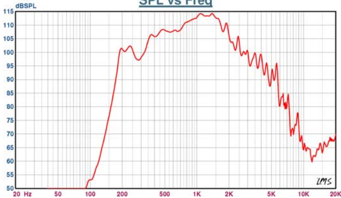
Sound pressure levels at 1W/1m with DS-100 driver
