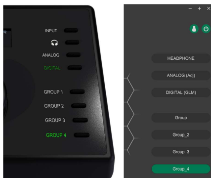
Fig. 8. The four GROUP keys select and activate (left) the first four Group settings in the GLM software user interface (right).
