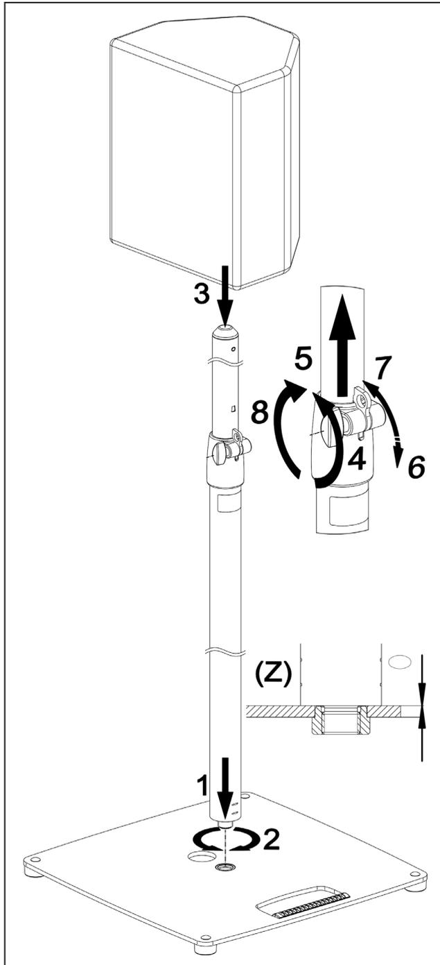
2.) Mount the tube combination on the base
