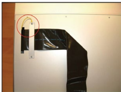
Fig 2-14 : Mixer Bus Cable Screen Connection.
